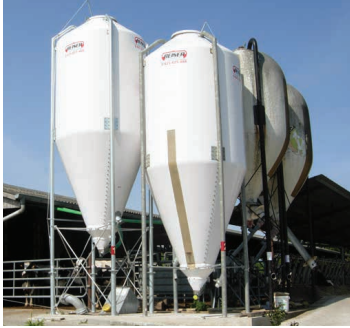
Silo supplying a milking robot, by flexible grain auger
